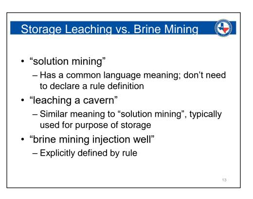
We have some common terms we use when referring to the process of removing salt by dissolution from a salt structure.
