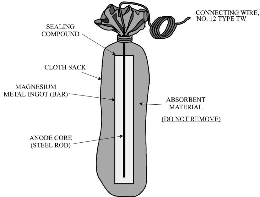
**Sacrificial protection** means the reduction of corrosion of a metal (usually steel in a gas system) in an electrolyte (soil) by galvanically coupling the metal (steel) to a more anodic metal (magnesium or zinc) (see FIGURE III-3). The magnesium or zinc will sacrifice itself (corrode) to retard corrosion in steel the pipe.
