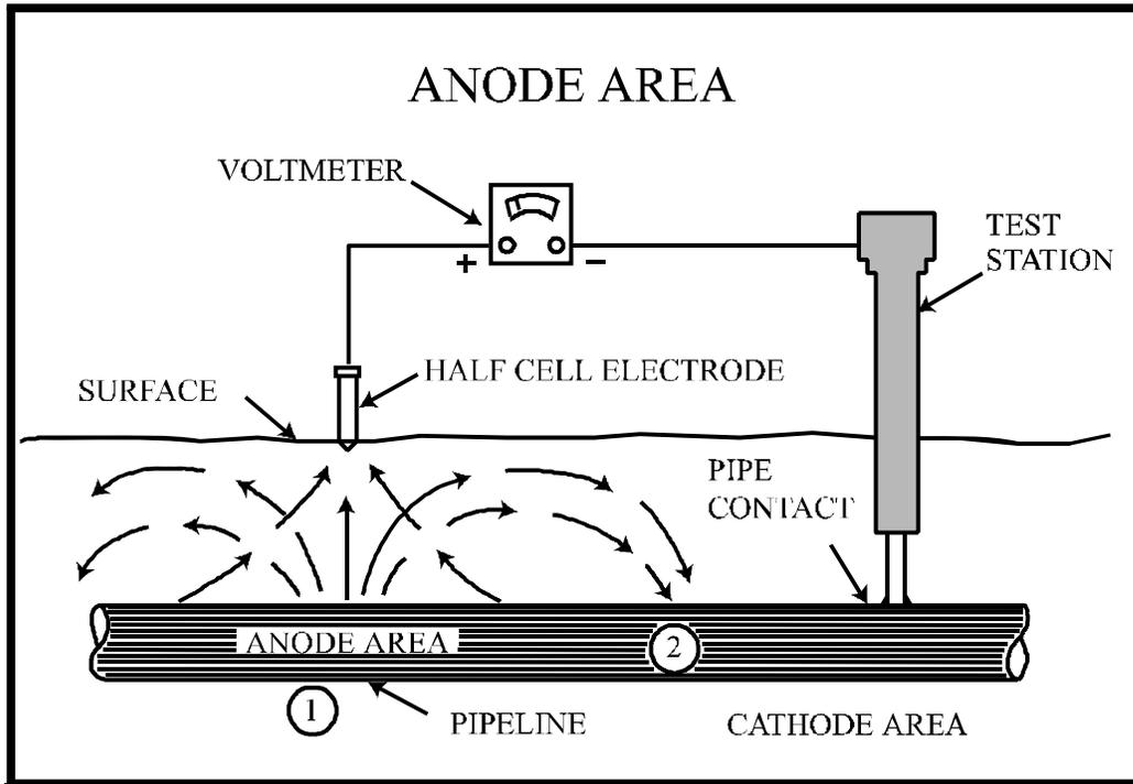
The voltage potential in this example is the difference between points 1 and 2. Therefore, the current flow is from the anodic area (1) of the pipe to the cathodic area (2). The half-cell is an electrode made up of copper immersed in copper-copper sulphate ( $\text{Cu-CuSO}_4$ ).
