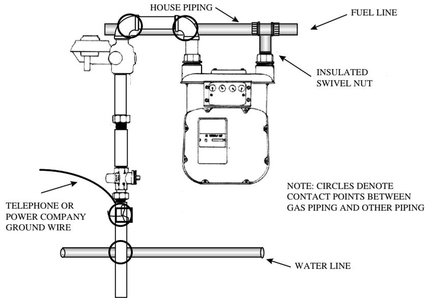
Unshaded piping shows Operators piping from service entry to meter insulator at location shown on sketch above. Shaded areas show house piping, electrical cables, etc.
