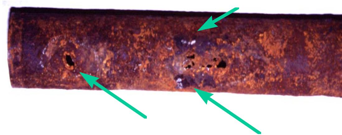
An example of bare steel pipe installed for gas service. Note the deep corrosion pits that have formed. Operators should never install bare steel pipe underground. Operators should use either polyethylene pipe manufactured according to ASTM D2513 or coated steel pipe as new or replacement pipe. If steel pipe is installed, that pipe must be coated and cathodically protected.
