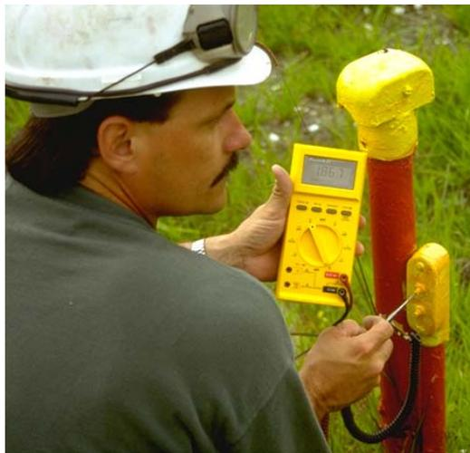
This is a pipe-to-soil voltage meter with reference cell attached. This is a simple meter to use and is excellent for simple "go-no-go" type monitoring of a cathodic protection system. If meter reaches at least -0.85 volt, the operator knows that the steel pipe is under cathodic protection. If not, remedial action must be taken promptly. **NOTE:** Be sure to take into consideration the voltage drop.
