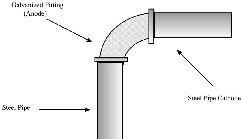
The galvanized elbow will act as an anode to steel and will corrode. Do not install galvanized pipe or fittings in system, if possible.
