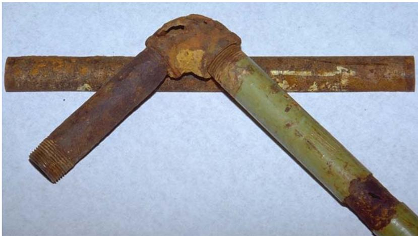
An example of a main which was buried without a coating or wrapping at the service connection. This corrosion problem could have been avoided by properly coating and cathodically protecting the pipe.
