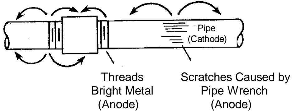
**(Corrosion caused by dissimilar surface conditions.)**
