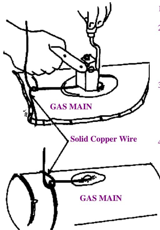
1. Loop wire as shown to avoid strain on bond.
