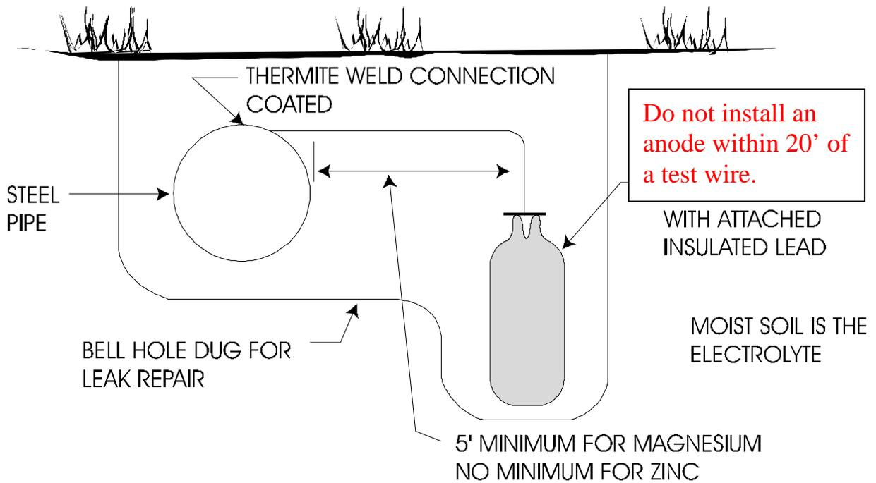
Zinc and magnesium are more anodic than steel. Therefore, they will corrode to provide cathodic protection for steel pipe.
