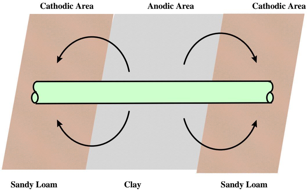
A corrosion cell can be set up when pipe is in contact with dissimilar soils. This problem can be avoided by the installation of a well-coated pipe under cathodic protection.
