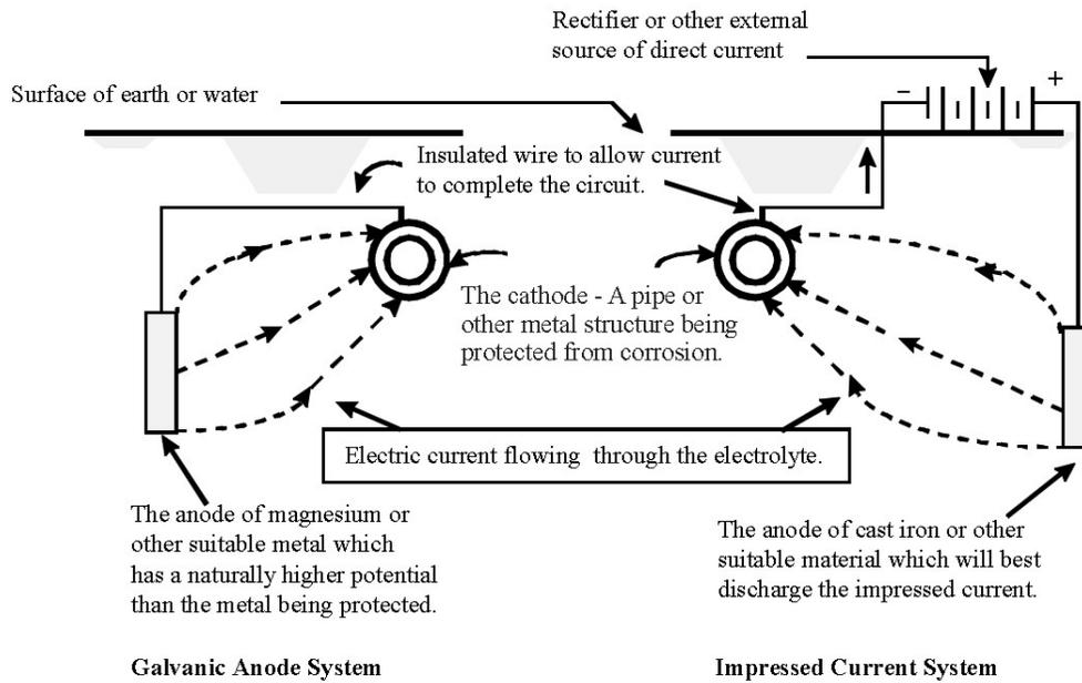
Any current, whether galvanic or stray, that leaves the pipeline causes corrosion. In general, corrosion control is obtained as follows:
