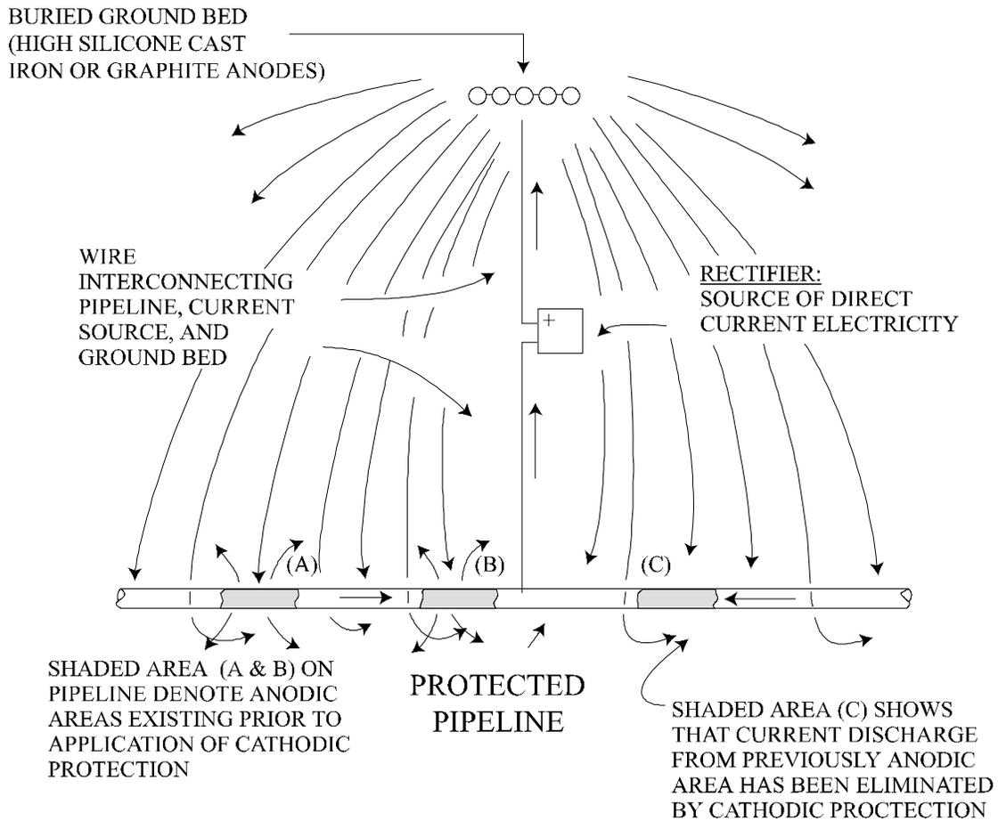
This illustrates how cathodic protection can be achieved by use of a rectifier. Make certain the negative terminal of the rectifier is connected to the pipe. **NOTE:** If the reverse occurs (positive terminal to pipe), the pipe will corrode much faster.
