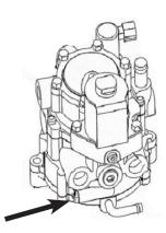
On the Aisan®, remove the 12mm head drain. Some applications have an extended drain fitting for easier access.
