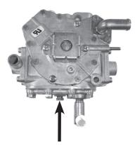
On the NIKKI®, remove the 12mm hex drain located at the very bottom of the vaporizer.
