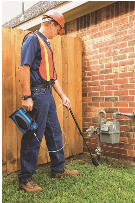
Figure IV-6: Checking a Gas Meter For Leaks With a Hand-Carried Infrared Optical Instrument.
